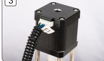
Insert the print head motor line 插入打印头电机线
