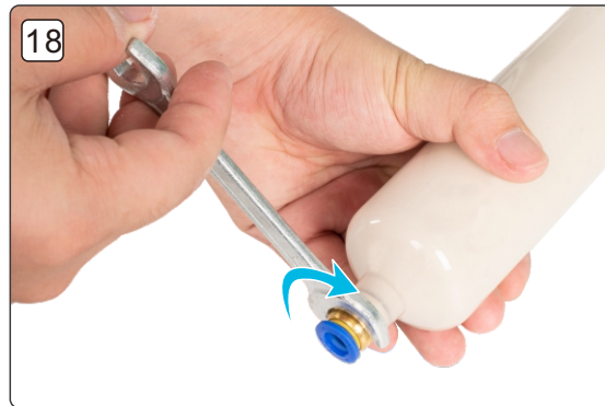
Tighten the pneumatic coupling with a wrench 使用扳手拧紧气动接头
