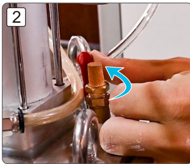
Pull up the material discharge switch 向下装卸料放气开关
