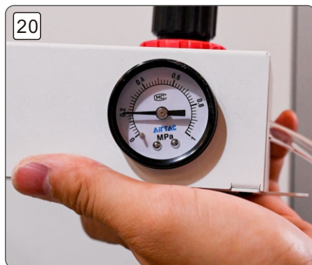
20 Adjust the air pressure to 0.2 调整气压至0.2
