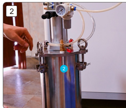
Take out the material barrel 拿出料筒
