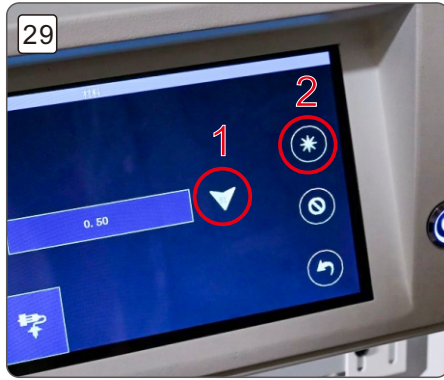
First click on icon 1, then click on icon 2 to extrude the clay 先点击图标1, 再点击图标2, 挤出陶泥
