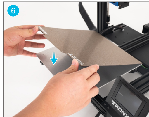
Align the hot bed and paste it 对齐热床贴下去
