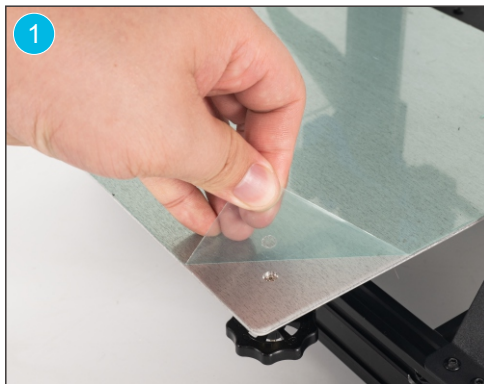
Tear off the protective film on the printing platform(hot bed) 撕开热床上的保护膜
