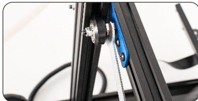
Use wrench to adjust the tightness of eccentric nut 使用扳手调整
