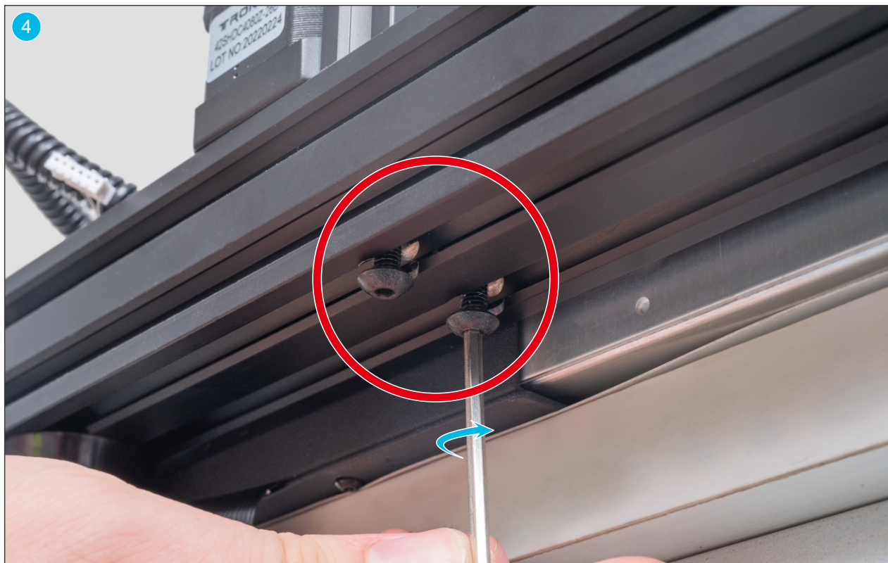
After inserting another M5*45 screw, tighten the two screws with a wrench 插入另一颗M5*45螺丝后,使用扳手拧紧两颗螺丝
