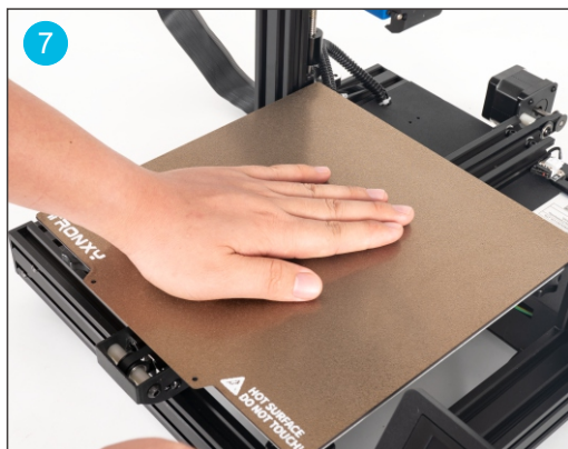
Press it with your hand to make the sticker stick to the hot bed 用手按压一下使贴纸粘紧在热床上
