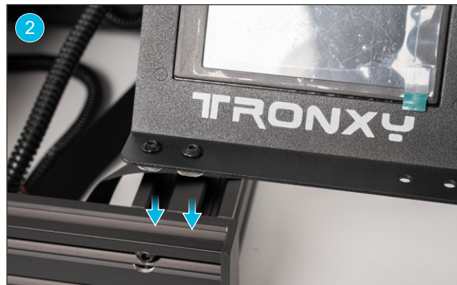
Put the boat nut into the groove 将船型螺母放入凹槽内
